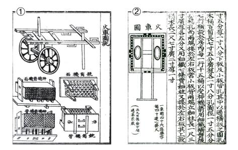
**Figure 2b.** Structure of *Hwacha* ① *Singijeon-Hwacha* launching 100 arrows ② *Hwacha* used in the *Haengju* Mountain Fortress Battle in 1592
