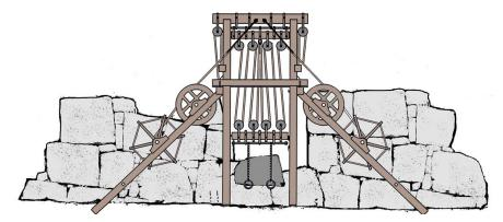
Figure 6a. Geojunggi was used in the construction of fortress walls
